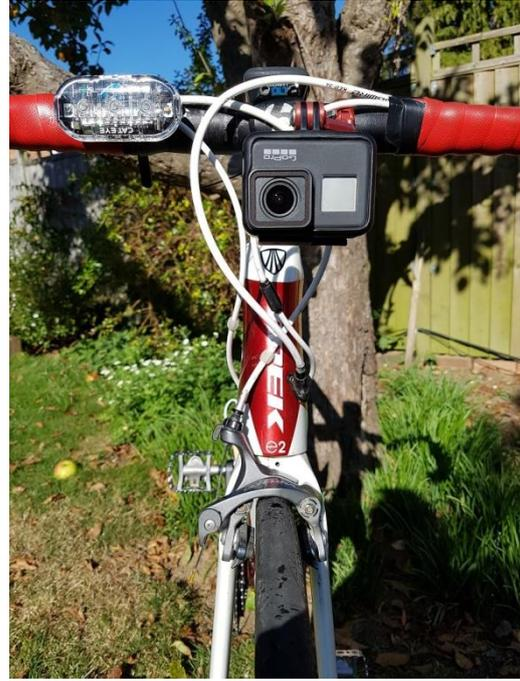
Adjust the camera's tilt on the mount so that the far horizon (eg the end of a long, level street) is centred vertically in the viewfinder.
